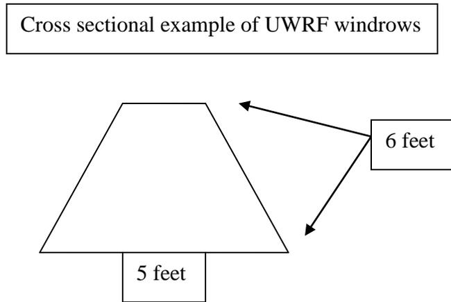
**Figure 1** Picture reference to windrow shape.
