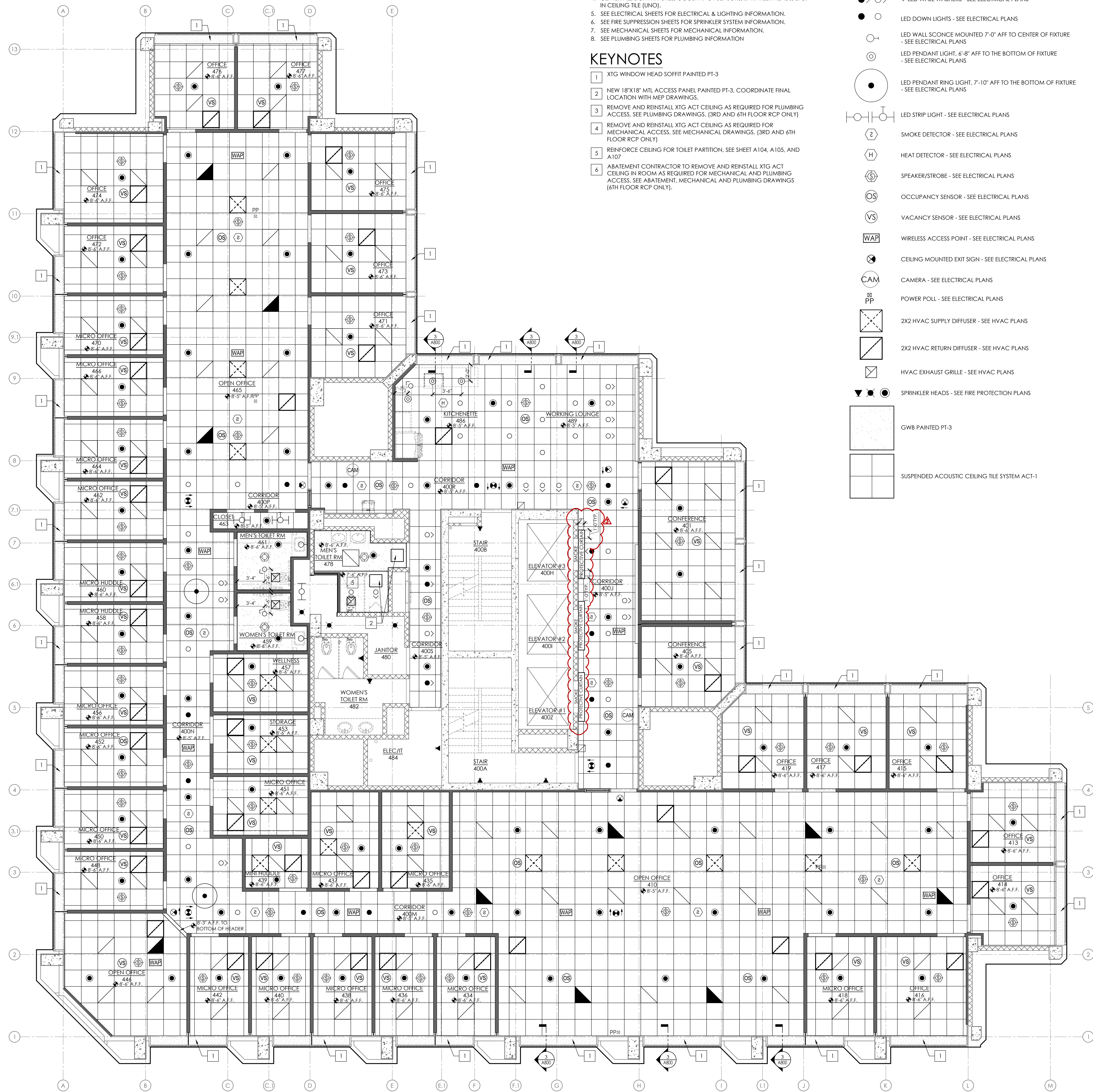
1 4TH FLOOR REFLECTED CEILING PLAN 3/16" = 1'-0"
