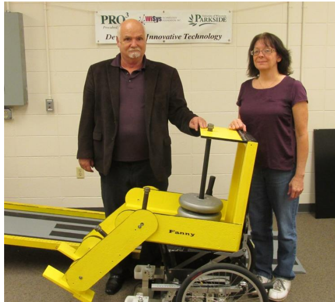
Weighted test dummy per ASTM standards. Students named it "Fanny."
